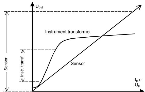
**Fig. 5** Linear range for instrument transformer and sensor
