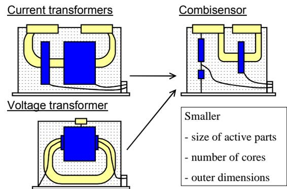
**Fig 11** Size of instrument transformers and sensors
