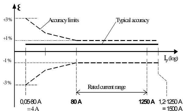
**Fig 7** Rated primary current range, accuracy limits and accuracy curve for a current sensor
