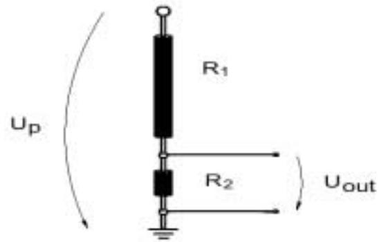
Fig. 2 Resistive voltage divider
