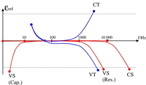
**Fig 10** Frequency response for current transformer (CT), voltage transformer (VT), current sensor (CS) and voltage sensor (VS)
