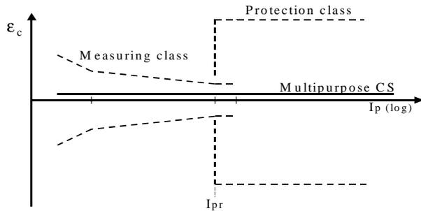
**Fig. 8** Accuracy limits for a multipurpose current sensor and a typical accuracy curve
