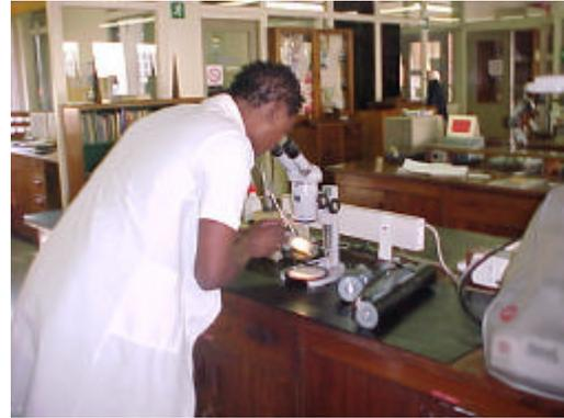
Figure 3: Routine microscopic examination of high voltage cable samples
