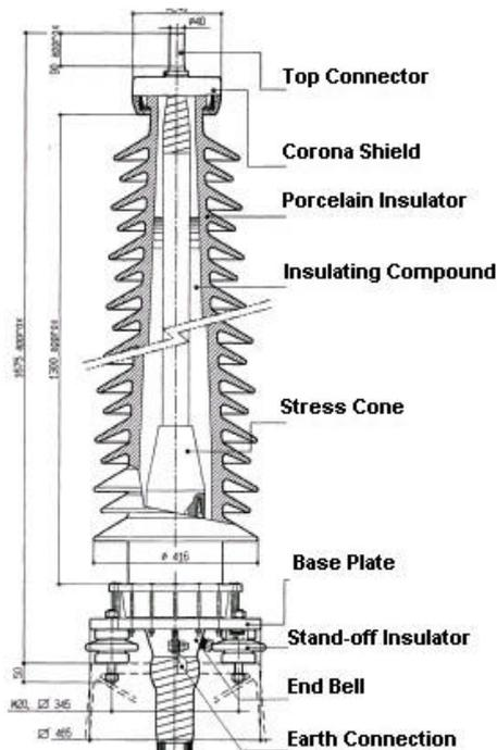
Figure A-1:132kV Outdoor Porcelain Sealing End
