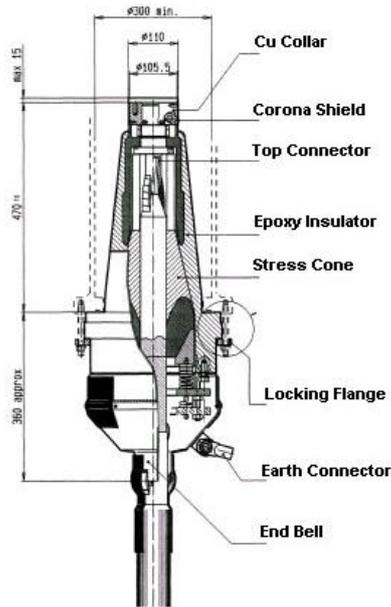
Figure A-3: 132kV SF6 Immersed Dry-Type Sealing End
