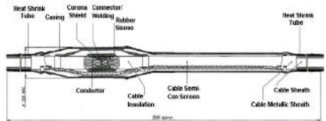
Figure A-4: Premoulded Straight Joint for extruded cables with Cu or Al conductors
