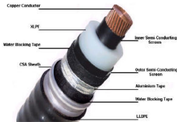
Figure 1: Components of the 1000mm<sup>2</sup> high stress cable manufactured by African Cables
