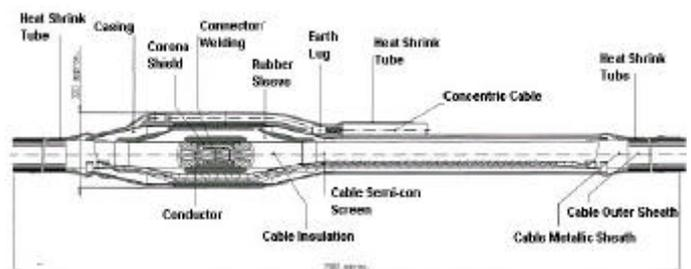
Figure A-5: Insulated Joint for extruded cables with Cu or Al conductors
