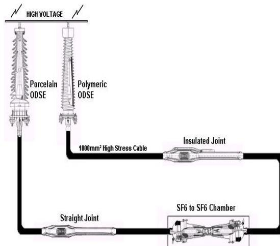
**Figure 5: Type Test loop on 132kV 1000mm<sup>2</sup> Cu high stress cable and accessories**
