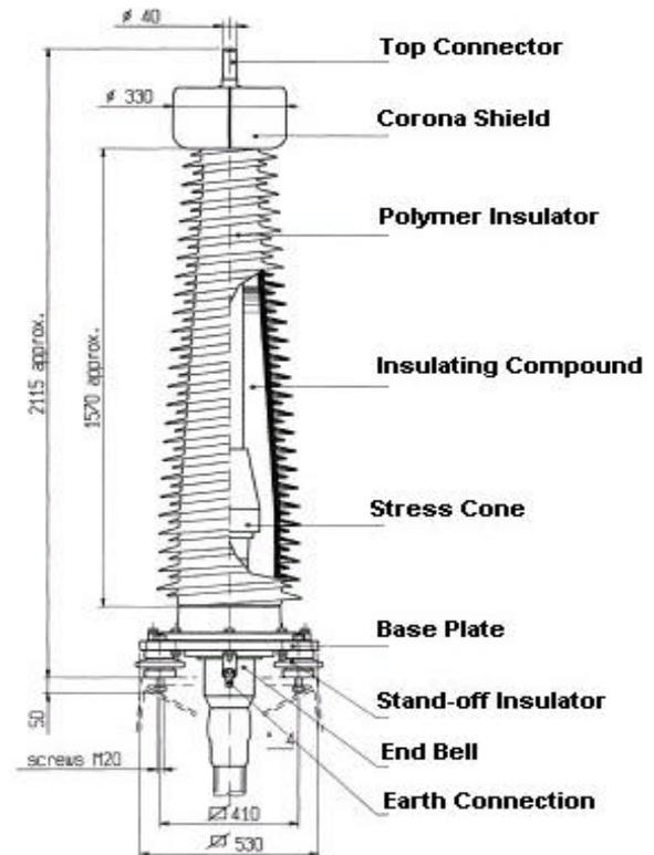
Figure A-2: 132kV Outdoor Polymer Sealing End
