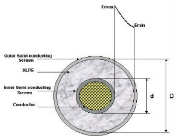
Figure 2: Electric Stress in a single core cable
