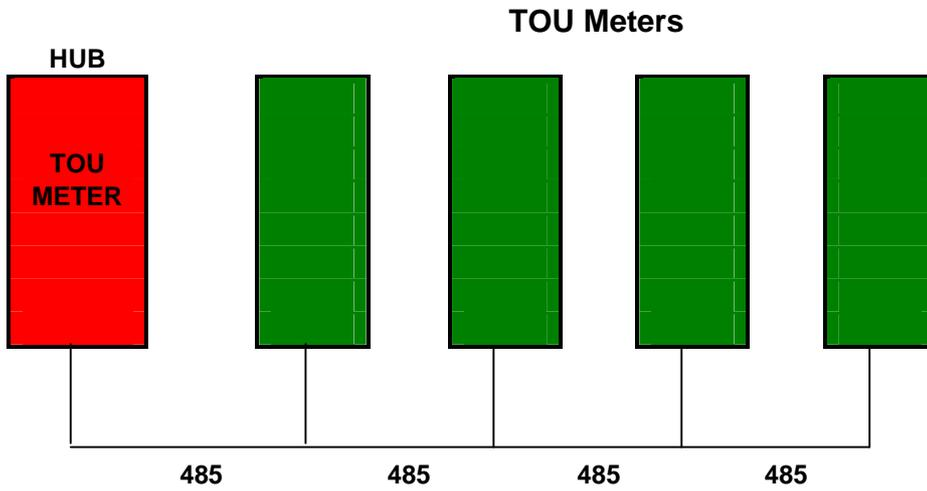
**RS485 Meters connected to "HUB"**
