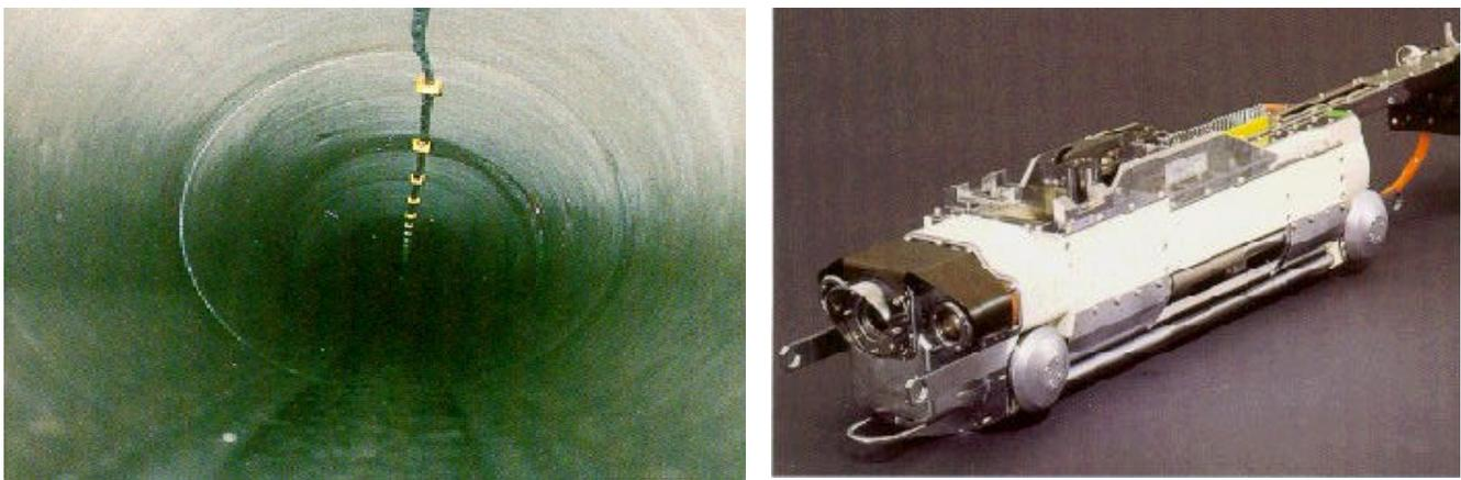
**Figure 2.** An example of the BerliKomm installation robot and an example of an optical fibre cable installed in Toronto.
