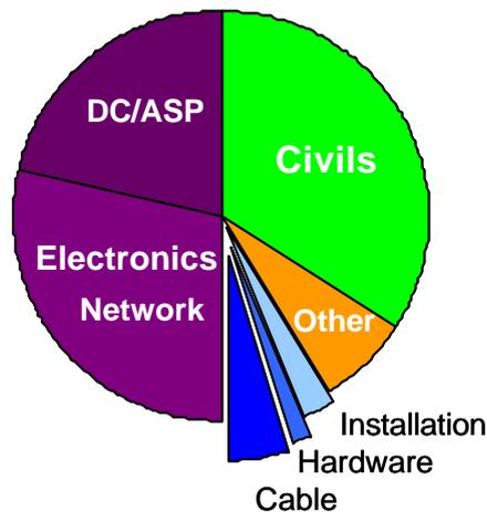
**Figure 1.** A typical breakdown of the cost involved in deploying an optical fibre cable network in an urban environment.
