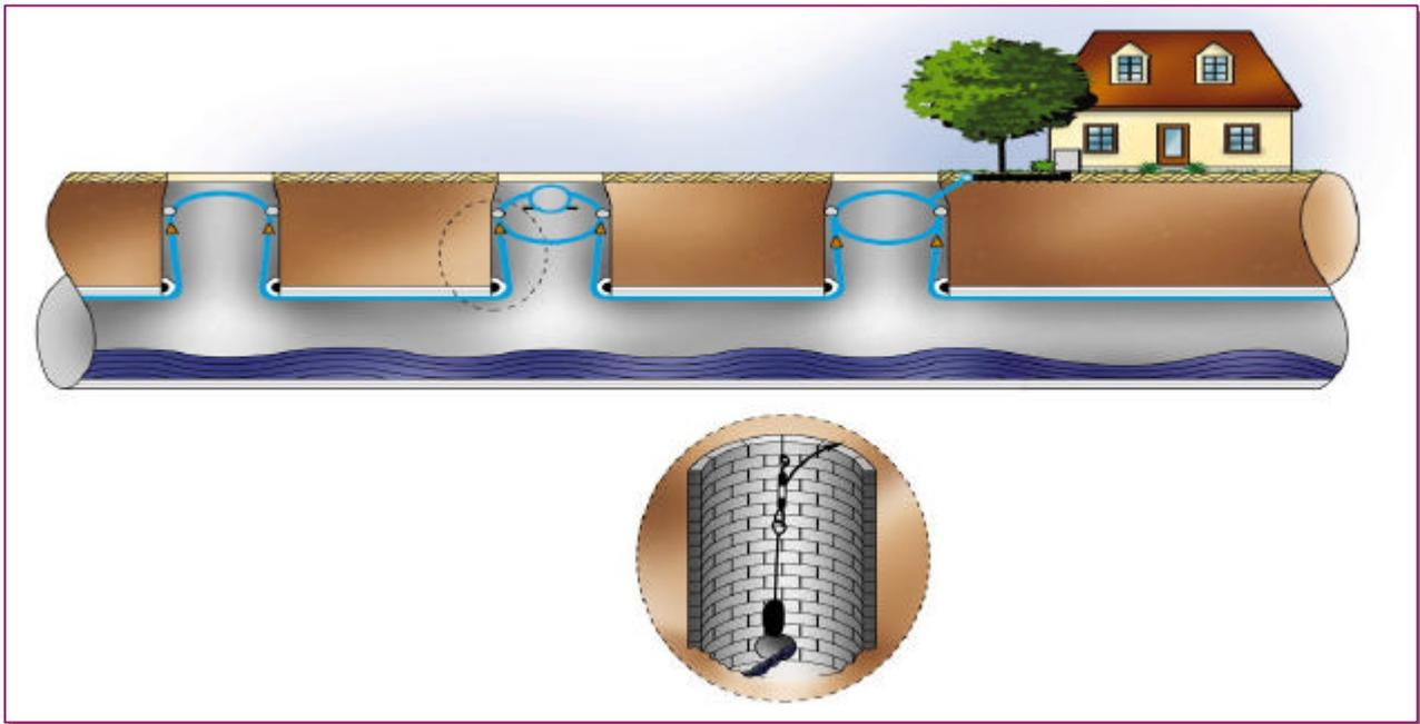
**Figure 4.** The MCS Drain solution from Corning Cable Systems negates the need for drilling into the sewer wall, as the cable is tensioned between two manholes over guide pulleys which are attached into the manhole wall. Using this installation technique, the possibility of contaminating the groundwater is negated as the integrity of the sewer or drain walling remains intact.
