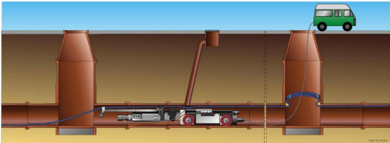
**Figure 3.** Corning Cable System's S.L.I.M. sewer solution uses a robot to attach the optical fibre cable to the roof of the sewer. With the S.L.I.M. technique the robot is controlled remotely above ground and it is possible to install multiple cables in a particular sewer run.
