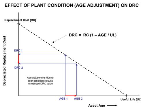
Figure 5: DRC method taking plant condition into account.
