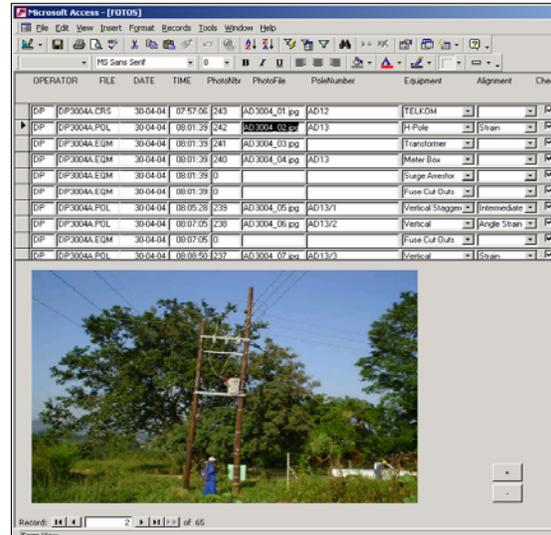
Figure 8: Example of database populated with field captured asset data, including an associated photograph.
