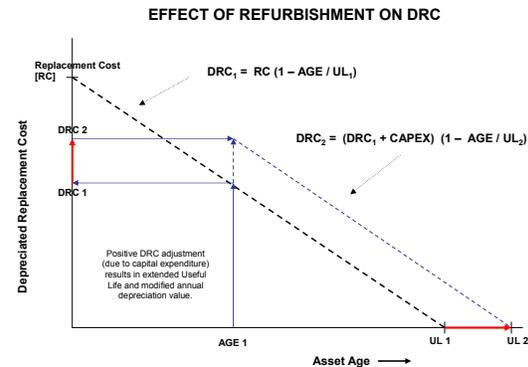
Figure 6: DRC method taking refurbishment into account.
