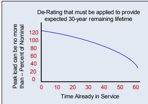
Figure 3-2: Transformer De-rating Curve
