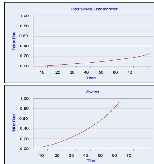
Figure 3-1: Equipment Hazard Rates
