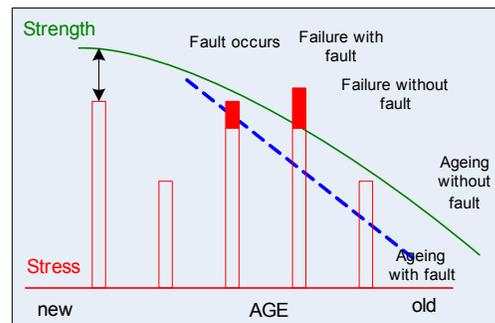
Figure 4-6: Transformer Failure Model
