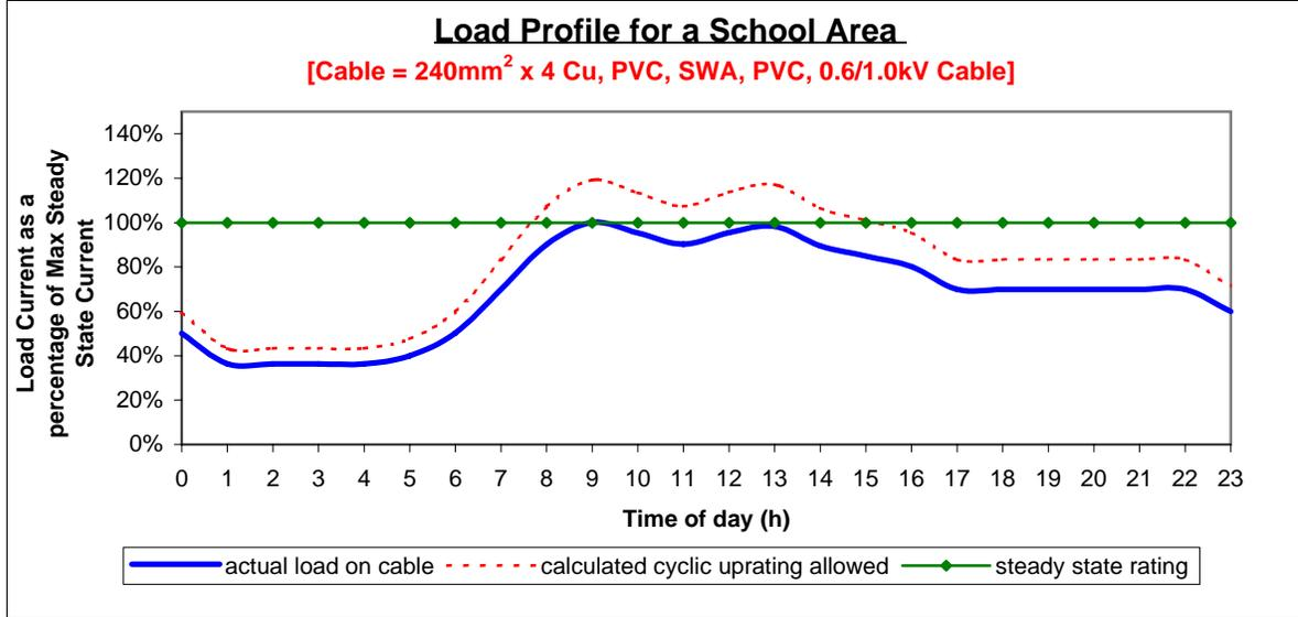
Figure 2: Load profile for a school area (dashed lines show calculated cyclic up-rating allowed on the cable)
