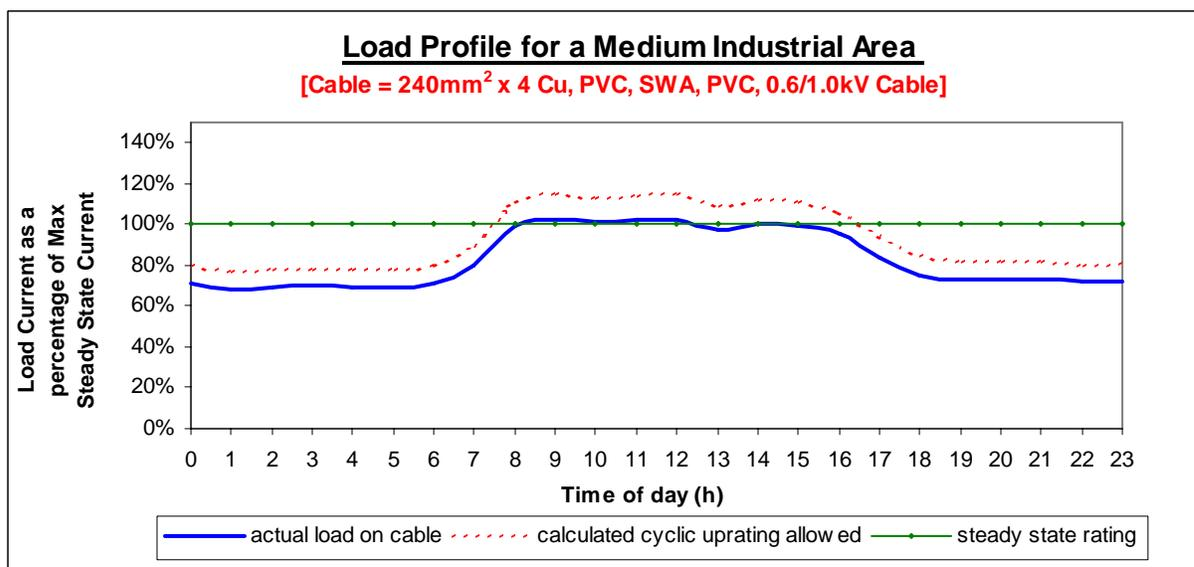
Figure 1: Load profile for a medium industrial area (dashed lines show calculated cyclic up-rating allowed on the cable)
