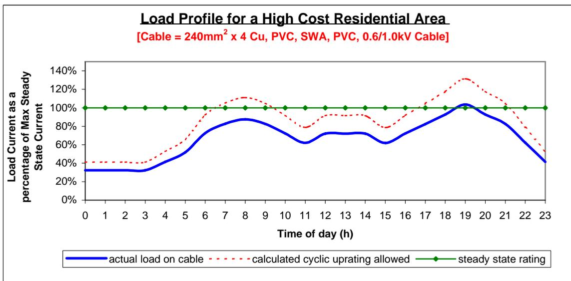
Figure 5: Load profile for high cost residential area (dashed lines show calculated cyclic up-rating allowed on the cable)
