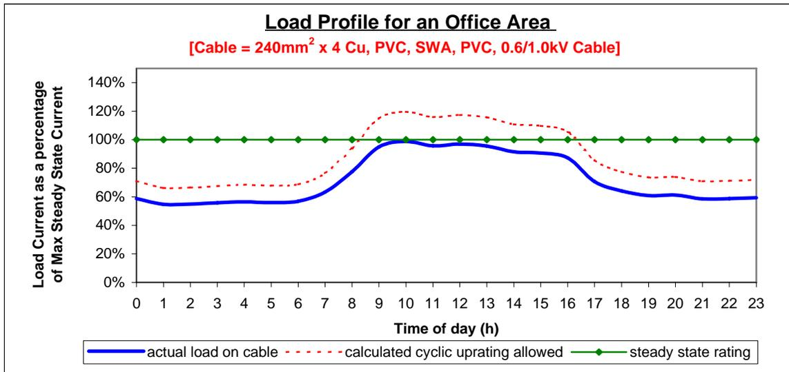
Figure 4: Load profile for an office area (dashed lines show calculated cyclic up-rating allowed on the cable)
