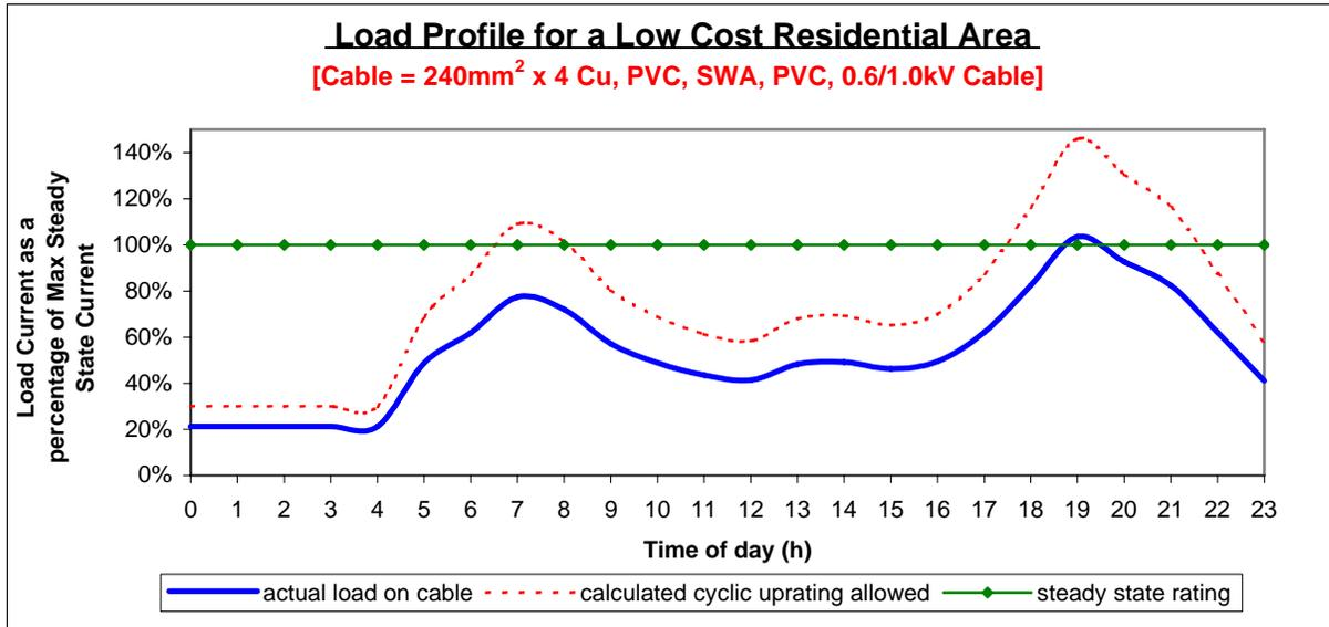
Figure 6: Load profile for low cost residential area (dashed lines show calculated cyclic up-rating allowed on the cable)
