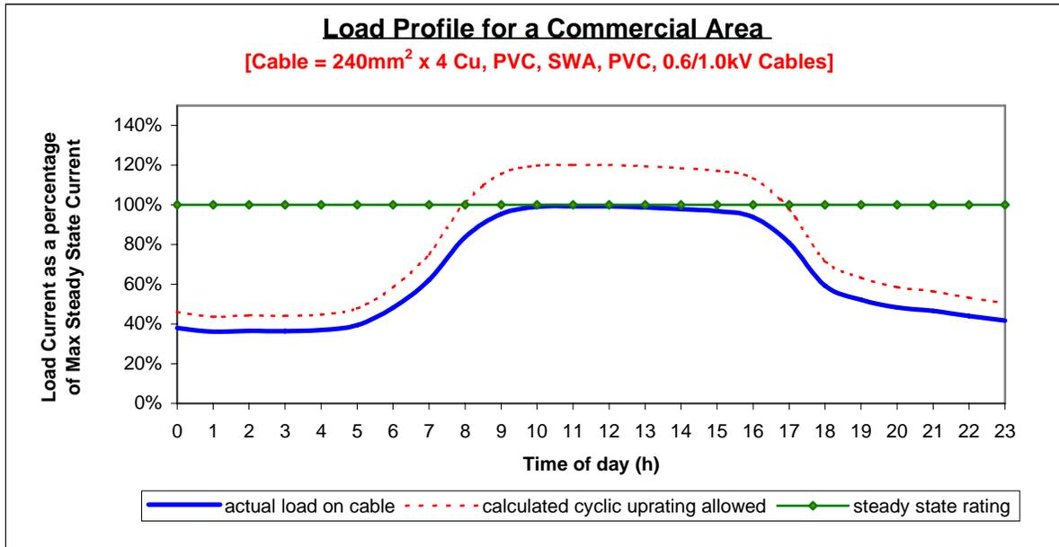
Figure 3: Load profile for a commercial area (dashed lines show calculated cyclic up-rating allowed on the cable)
