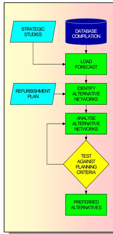
Figure 3: The basic process of network expansion planning.
