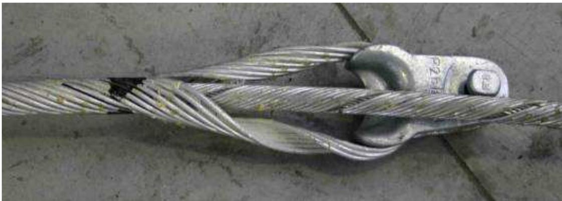
**Figure 4.** A typical helically formed spiral dead-end and protection rod configuration used in the type test.
