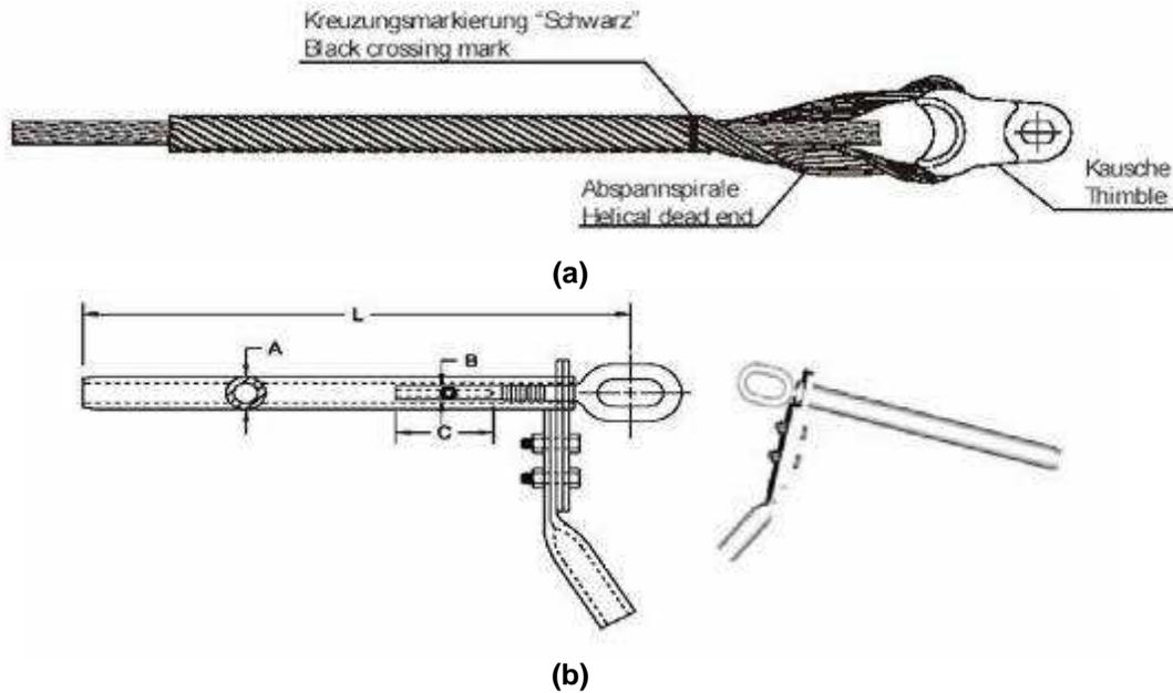
**Figure 1.** (a) Conventional helically preformed spiral strain assembly (b) an example of a crimp type compression fitting.
