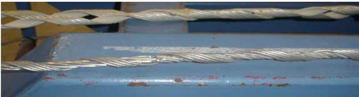
(c) Application of the aluminium conductive rods and armour rods to electrically bridge the section of aluminium layer removed. Note that the lay direction of the ACSR aluminium layer and the armour rod is in the same direction to maximise contact between the two layers.
