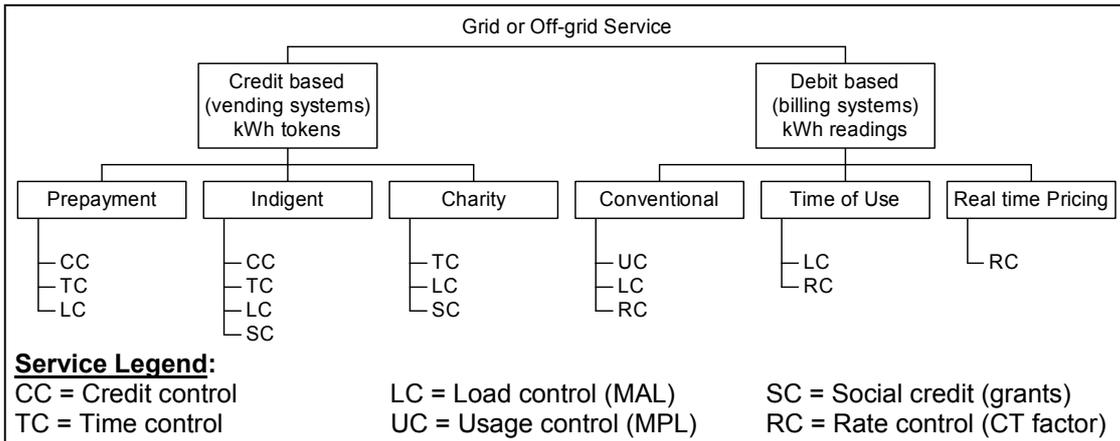
**Figure 3: Service capabilities of a typical multi-service meter**
