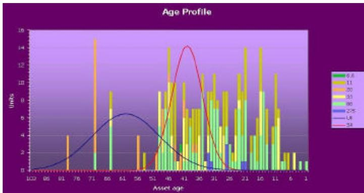
Here the assets under the different curves can be seen clearly and from field experience it is clear that these assets do not need replacement. This data has been taken from age information for the utilities power transformers, supplied to us, up to and including data for 2005.
