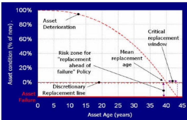
Diagram 4 shows the critical replacement window and the risk zone for "replacement ahead of failure policy".
