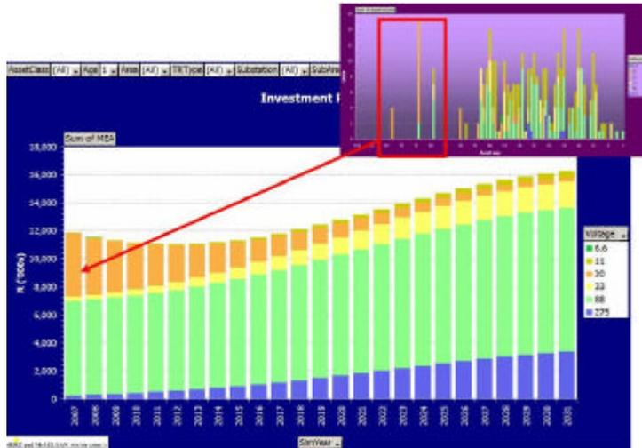
Diagram 5 shows the Investment Profile for the Asset Class of Transformers for a South African utility. The profile shows a present backlog of refurbishment being units still in service that have now entered the “Risk Zone”. (Refer inset) This does not mean that the units are unsafe or that a catastrophe is waiting to happen, but it does mean that the units should be inspected, their condition verified and the appropriate action initiated.
