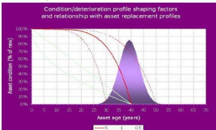
In Diagram 2b we have shown the Deterioration Curve and the relationship to the Asset Replacement Profile. Asset Managers experienced in using this type of modelling tool can combine their field knowledge of the Asset Class to accurately match the real conditions within the model.
