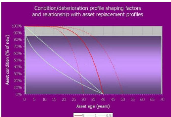
Diagram 2 shows a deterioration curve in red with a deviation of  $\pm 10$  years. This asset has initially a slow rate of deterioration which increases as it ages. The blue line to the left is the curve for a different asset type that initially deteriorates quickly then slows down as it ages. The straight line in blue is the standard normally used by the accountants.
