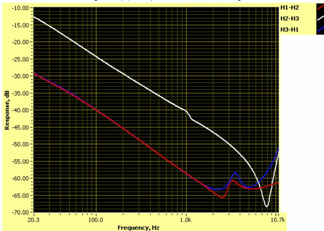
These are the responses of the HV and LV winding of the same transformer. There is clearly a significant difference in the White phase when compared to the other two phases. This is a result of a shorted turn failure. A shorted turn has the effect of creating an imbalance in the reluctance on one of the core limbs (in this case the white trace), which produces this characteristic change in the low frequency response. Excitation current and ratio test supported this diagnosis.
