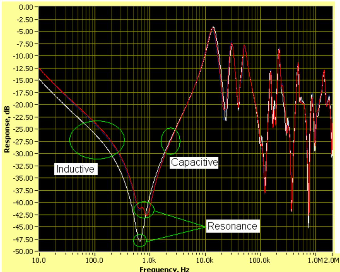
Figure 2: Frequency Response of a sound transformer
