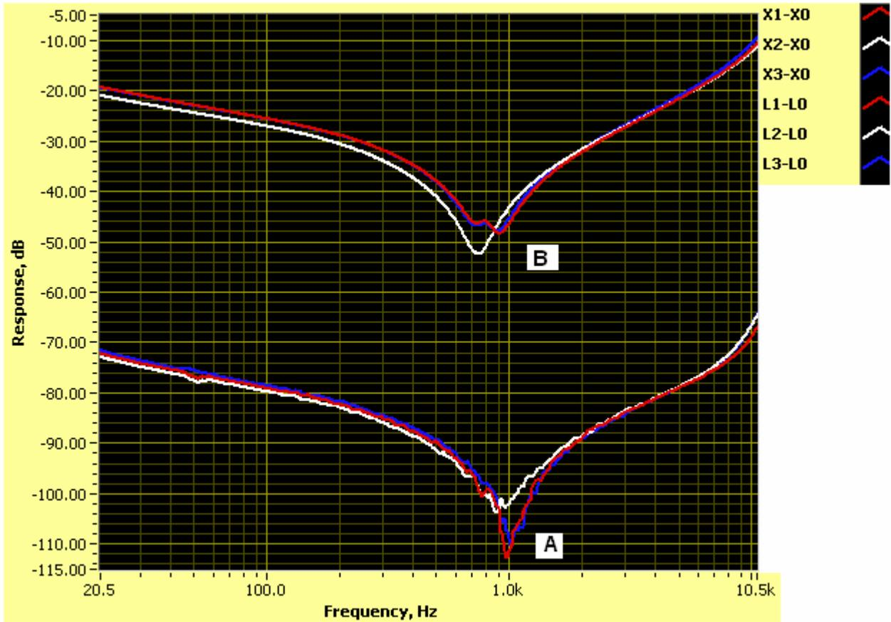
Figure 4 (A) shows the LV winding response of a multiple grounded neutral and Figure 4 (B) shows the response after the transformer was repaired. The comparison of the two responses shows a significant difference in the starting dB values. This difference in the dB or vertical shift in response A is attributed to the change in the resistance of the transformer under test.
