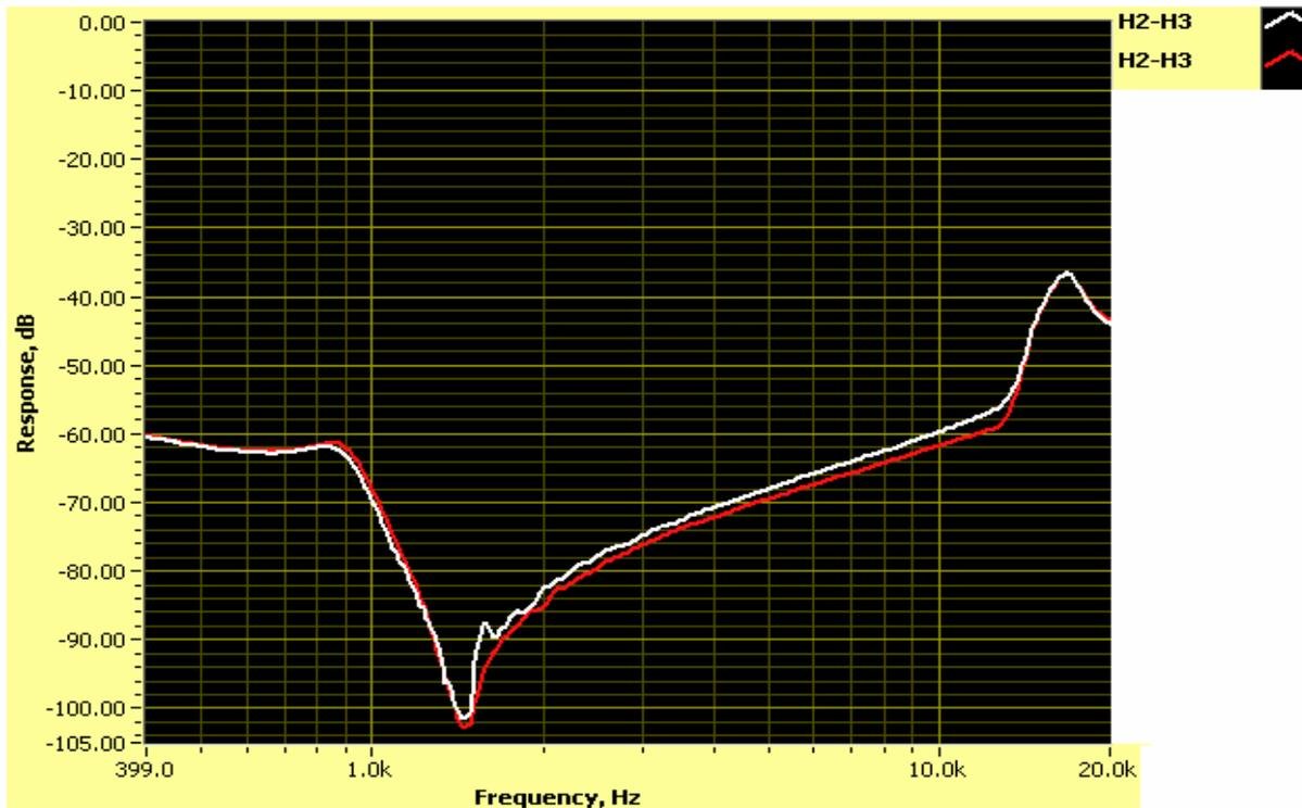
Figure 6 (A) and (B) shows the response of the middle phase with (White trace) and without (Red trace) the extra core earth. Differences were noted on all three phases but the greatest difference was noted on the middle phase. Figure 6 (B) shows a difference in the capacitance response from about 1,5 kHz to 14 kHz. Further, the White trace has a resonance frequency at 1,6 kHz which is absent in the Red trace. This creation of a new resonance frequency is clearly a cause of concern.
