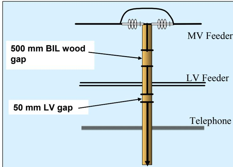
Figure 7: Optimal bonding and earthing of shared structures in densely populated areas with high lighting density.
