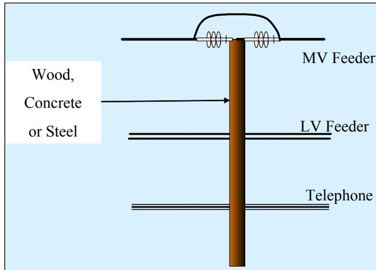
Figure 6: How do you bond and earth a wood pole structure shared by MV, LV and other services safely and with the lowest network risk?
