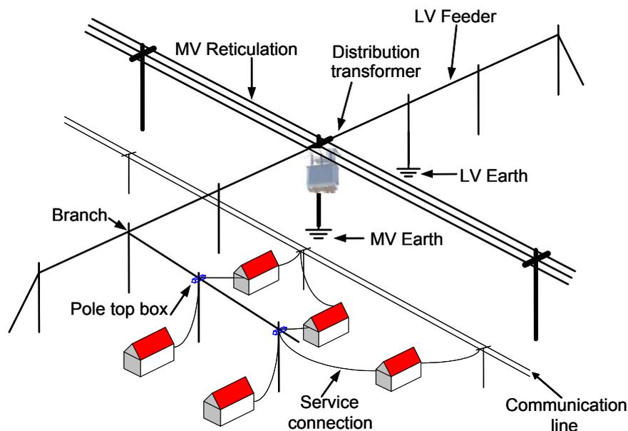
**Figure 1.** Ensuring safety and optimum performance: The environment in which a distribution supply system operates includes the service to customer and his installation (home), and the exposure of the public (in the street), this is impacted by environmental factors such as pollution, lighting, accidents, vandalism, other services etc. (Artwork: A Dickson.)
