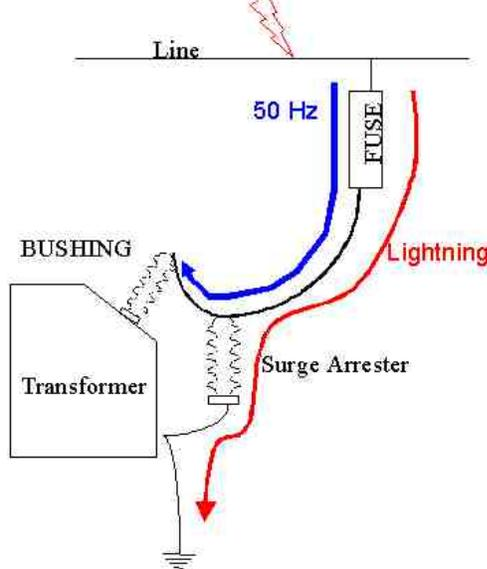
This configuration performed satisfactory under normal 50hz conditions but when it was exposed to over voltage occurrences such as lightning, the vulnerabilities exposed itself in excessive fuse blows and pole mounted transformer losses.
