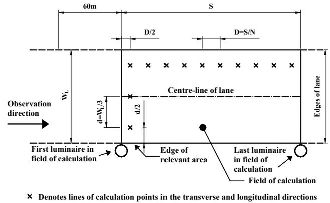
Figure 7 - Position of calculation points in a driving lane
