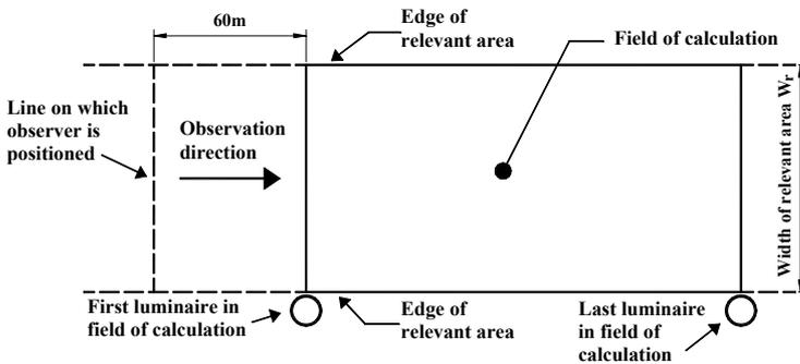
Figure 6 - Field of calculation for carriageway luminance.
