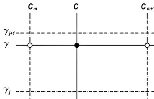
Figure 2 - Angles required for linear interpolation of luminous intensity.
