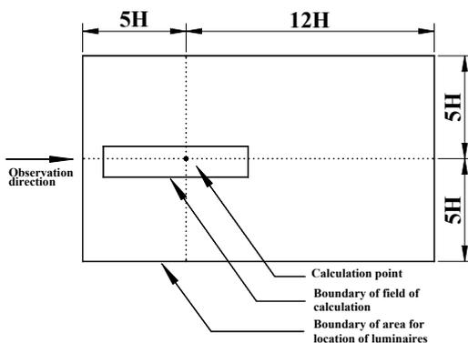
Fig. 8 - Luminaires which may contribute to luminance at calculation point.
