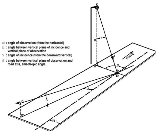
Figure 5 - Angular relationships for luminaire, observer and point of observation.
