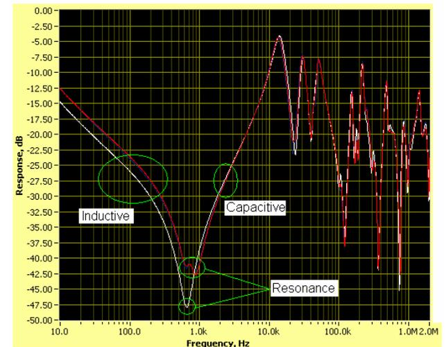
Figure 2: Frequency Response of a sound transformer
