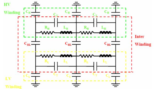
Figure 1: Simplified equivalent circuit with lumped RLC components
