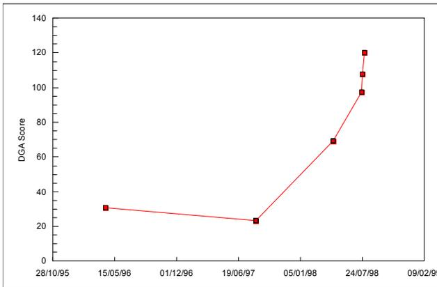
Figure 2: DGA score for core earth fault
