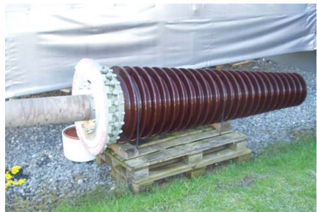
Fig. 19: 245kV RIP bushing stored outside
