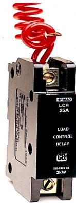
These clip mounted “Load Control Relays” (5) are designed to control any non-essential load. They are designed to fit easily into standard residential, commercial or industrial panel boards and operate on the principle of monitoring any peaking loads (of which cooking loads are a prime example) and shedding any non-essential loads. It becomes apparent the any load shedding is effectively under the control of the user through their own electricity usage patterns and actions.
