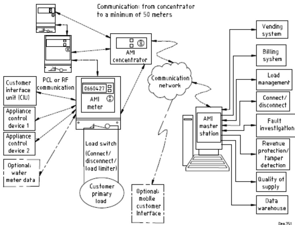
Figure 2 — Illustration of a typical AMI utilizing a concentrator
