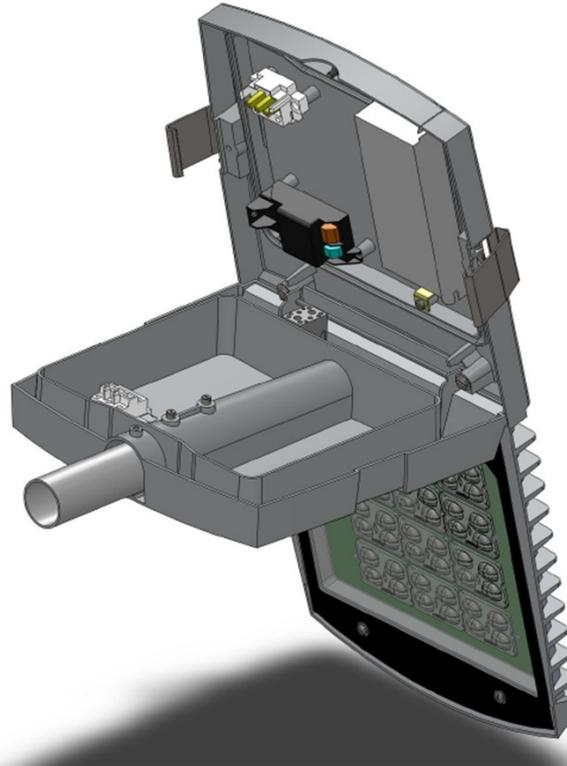
Optical compartment IP66 *LED Safe*® engine completely sealed by an extra-clear glass or PC protector for an optimal luminous flux and lower lumen depreciation. The concept of the photometric engine is consistent with the *FutureProof* principle. It will be able to be replaced on site with no tools required, taking advantage of future technological developments.
