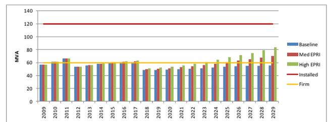
Figure 15: Example where Network Expansion plan needs revision to accommodate load growth
