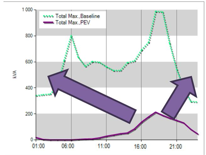
Figure 18 Baseline load profile vs PEV component (2029) example
