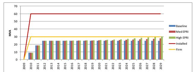
Figure 14: Example where additional load can be shifted to adjacent substations
