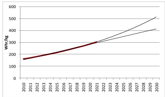
Figure 2 Battery energy density forecast
