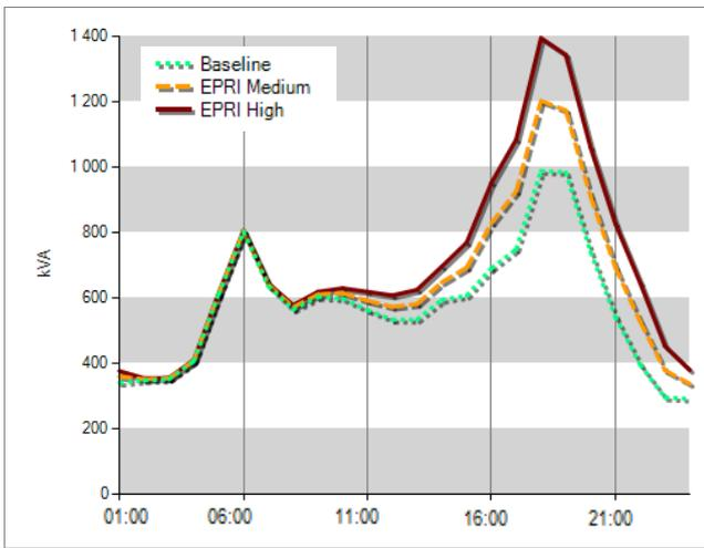
Figure 17 Uncontrolled MV load 2029 profile sample
