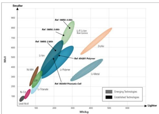
Figure 1 Energy densities for battery chemistries [ICCNexergy]
