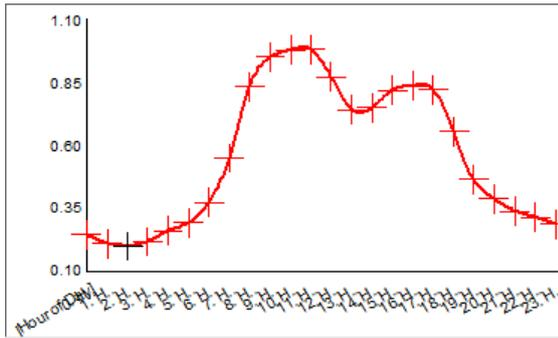
**Figure 4 - Light commercial /professional load profile with peak at 12pm**
