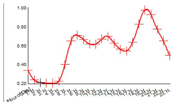
**Figure 3 - Domestic load profile with peak around 7pm**
