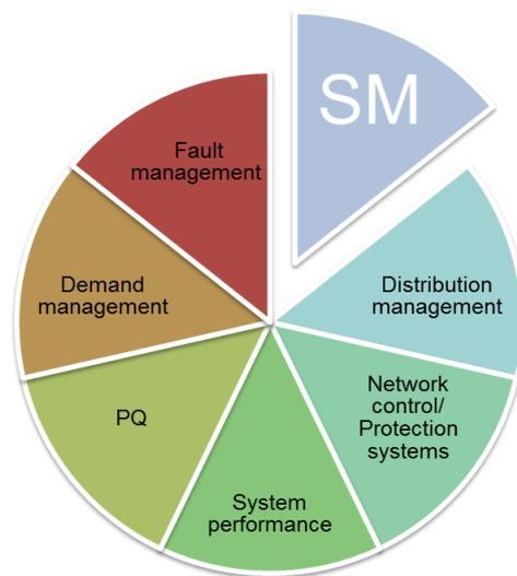
Figure 1: SG functional components
