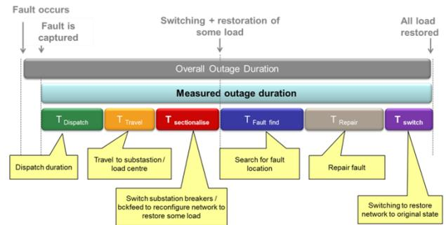
**Figure 3: Outage duration components associated with MV feeder outages**
