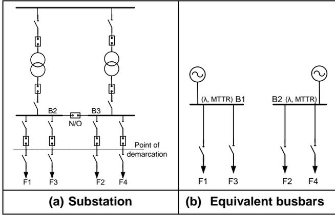
**Figure 1: Reducing a substation to a busbar with equivalent unavailability (adapted from [7])**
