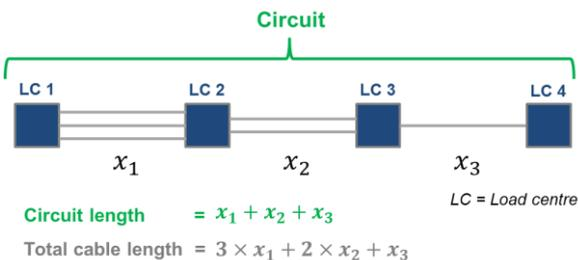
**Figure 2: Diagram illustrating cable exposure to common mode failures**
