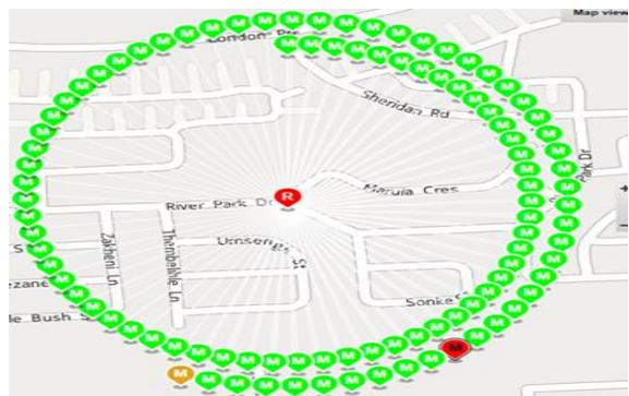
Figure 5: Data Concentrator Indicating one faulty meter
