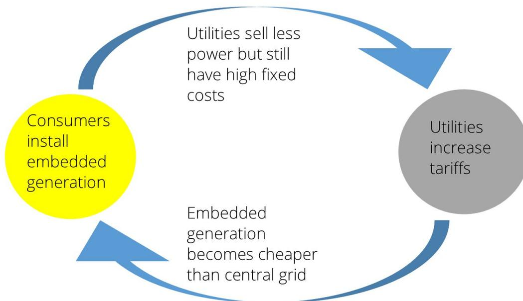
Currently, solar PV on its own (even with batteries to store energy at night) is unlikely to be a customer's sole source of generation. The reality is that most residential, commercial and industrial customers will not have the roofspace to generate 100% of their energy needs from solar. These will face a choice whether to continue purchasing from the grid or, if the tariff costs are too high, to consider an off-grid solution,
