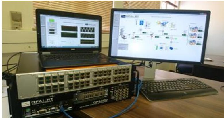
Figure 4: Hardware configuration of modelling in the loop
